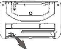
3.) Position the cover over the battery compartment and place the cord into the notch on back cabinet as shown.
